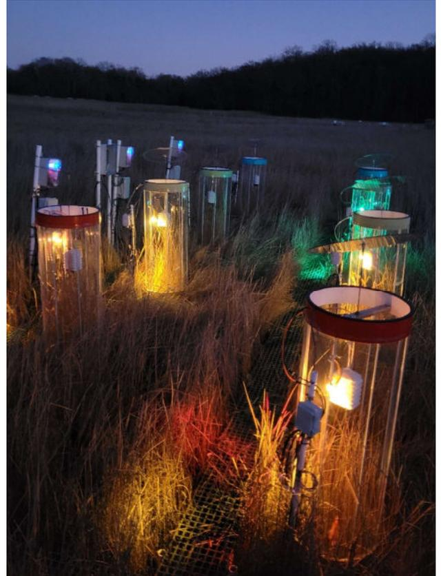
As part of our new Pathfinder project, we are seeking to fill three internships focused on advancing CO<sub>2</sub> and CH<sub>4</sub> gas flux chamber prototypes for use in remote settings. This work is important because it will expand the spatial and temporal range for which these types of instruments can be deployed, leading to better assessments of carbon flux into and out of the atmosphere.
